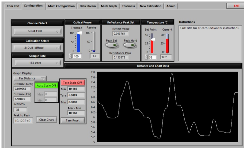
Figure 3.18: Optical Sensor Displacement Data Output in Philtec DMS Control Software (Courtesy of Philtec)
