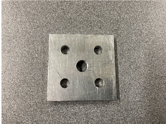
Figure 3.4: Machined Micrometer Bracket
