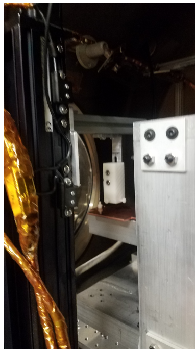
Figure 4.11: Mounted Damping system
