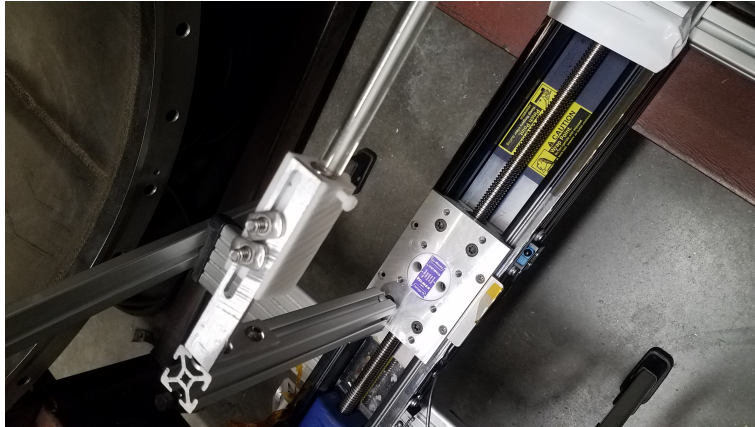
Figure 3.40: Magnet Support Slide attached to Linear Stage
