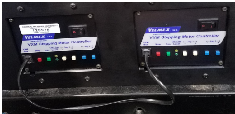
Figure 3.41: Velmex VXM Stepper Motor Controllers
